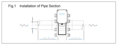
The reason for this procedure is to achieve a stable flow profile inside the pipe and by doing so, get a true reading. Please be aware of the fact that it is practically impossible to theoretically predict when the flow is stable after disturbances in the piping, so this must serve as a guideline only. The Monitor can give you a reading which is off from the calibration, if the straight runs are not within specifications.
