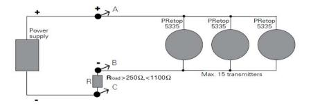
The outputs of max. 15 Flow Monitors (transmitters) can be connected in parallel for a digital HART® communication on 2-wires.
