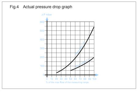
$\Delta \mathbf{p} = (\mathbf{Q}/\mathbf{Q} \max)^2 * 200$ and  $\Delta \mathbf{p} = (\mathbf{Q}/\mathbf{Q} \max)^2 * 550$  for turn down ratio of 1:2
